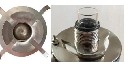
4. When the O-ring is seated, screw the knurled nut back on and tighten only by hand firmly. **Caution: Do not apply any thread tape, grease, or sealant as this will void the warranty. Overtightening the nuts may cause the thimble to crack.**
